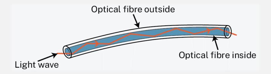
The light is reflected inside the optical fibre and moves along it to reach its destination.
